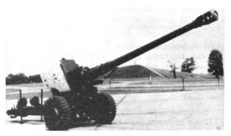
Figure 6-26, 122-mm field gun D-74. The D-74, with a range of about 23,900 m, can be rapidly shifted through a 360 degree traverse with the aid of a firing jack and the two large castor wheels on the trail.
